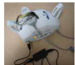
Figure 12E - Charger is connected to the lift. The indicator light on the charger will be ORANGE indicating that the lift is charging.
