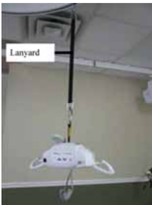
Figure 10A - Photo of lift hook connected to a P-440 lanyard first and then to the eyelet of the trolley.
