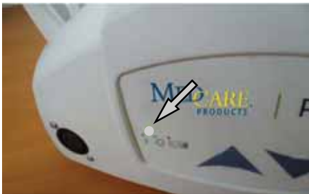
Figure 4B – The indicator light of the lift is normally off when not in use
