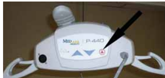
Figure 14B –RED emergency lowering button located on middle of the front of the lift.
