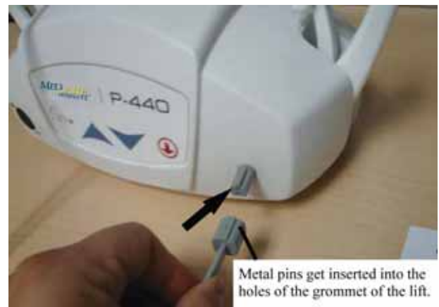
Figure 15B - Gray rubber airline being inserted into rubber grommet of lift. The ridges on both pieces are lined up. The metal ribbed pins are on the airline (within the shroud).
