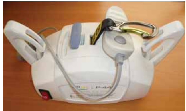
Figure 14C –RED Emergency stop switch located on the front left side of the lift.
