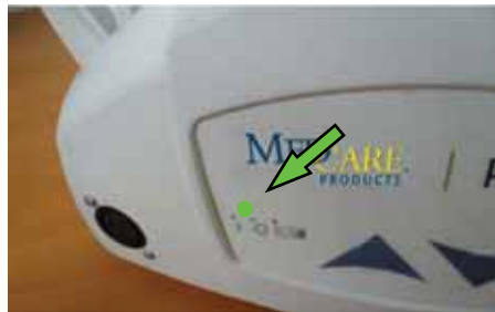
Figure 4C – When the lift has been turned ON, the indicator light will turn green
